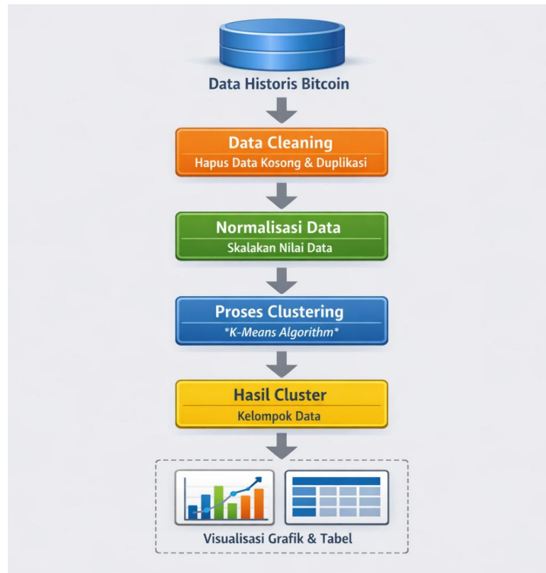
Gambar 2. Diagram Alur Proses Pengolahan Data
